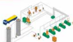
BCS series (Dry-Air Conveying System) 2.2 kw, 4 kw, 7.5 kw to 11 kw with "n" number of stations
