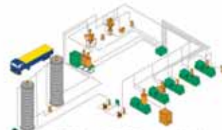
BCS series (Bry-Air Conveying System) 2.2 kw, 4 kw, 7.5 kw with "n" number of station
