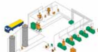
BCS series (Bry-Air Conveying System) 2.2 kw, 4 kw, 7.5 kw with "n" number of station
